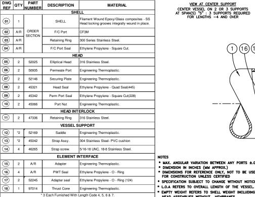
VIEW AT CENTER SUPPORT CENTER VESSEL ON 2 OR 3 SUPPORTS AT SPAN(S) "S" : 3 SUPPORTS REQUIRED FOR LENGTHS -4 AND OVER
