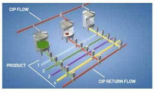
TANK IS BEING FILLED GAS VENTING GAS SUPPLY OR VENTILATION YELLOW: TANK IS BEING EMPTIED TANK IS BEING CLEANED SUPPLY OF CLEANING FLUIDS (CIP MEDIA)
